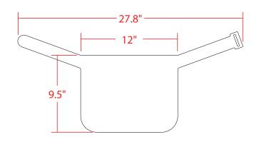
**Protective Face Shield**Assembled with velcro and padding
